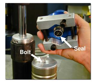
While pressing down on the tool body, tighten the clamps on the reservoir body evenly.
